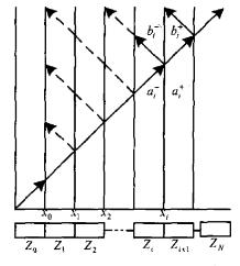
Fig.1 Lattice diagram analysis for cascaded transmission line
