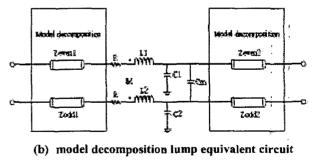
Fig.4 Lump equivalent circuit model
