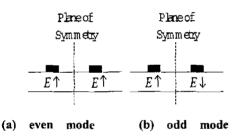
Fig.3 Even mode and odd mode excitation
