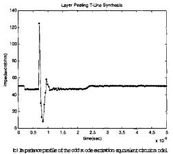
Fig.5 Impedance profile of even and odd mode excitation equivalent circuit model
