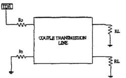
Fig.2 Couple lossless transmission line circuit
